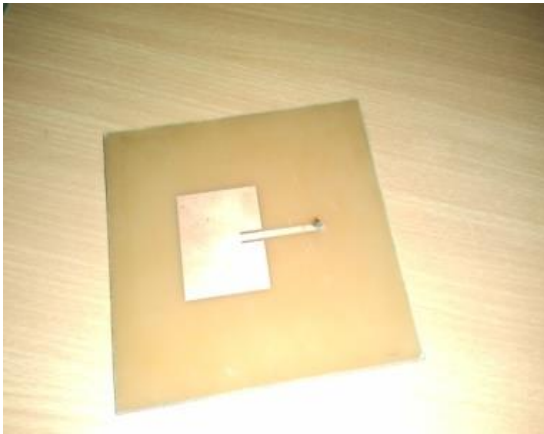
Fig 16. Microstrip patch antenna on PCB plate.
